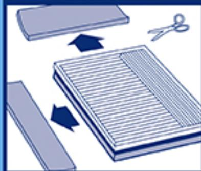
Using the old filter or slide-in screen as a guide, trim the filter pad to size. Fits sizes 15" x 24" and smaller.
