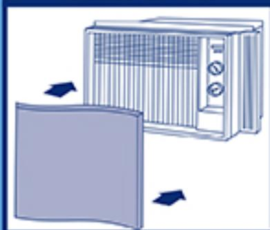
Removable grill: Install filter directly into grill and snap grill back onto A/C.
