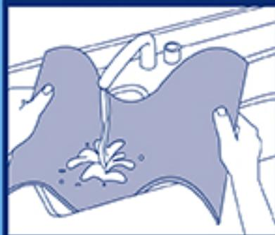
Clean every 30 days to prevent damage to air conditioner. Rinse with cold water to remove dirt. Squeeze out excess water.
